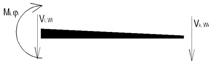
Figure 9 Sign convention for moments, shear forces, displacements, and rotations for the stiffness matrix
