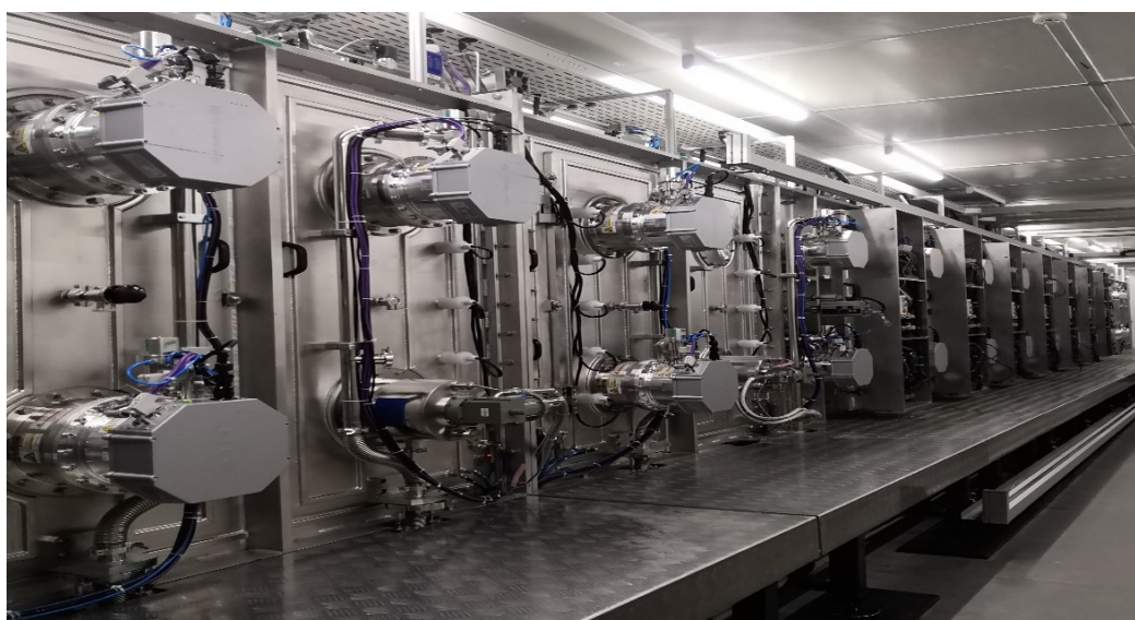
Figure 2. Leybold Optics Inline A1100V4 DC magnetron sputtering system.
