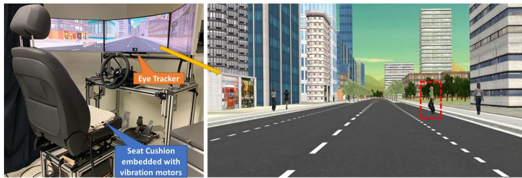
Figure 1. Driving simulator and a mid-block crossing pedestrian scenario. Left: custom-built driving simulator. Right: screenshot of the center screen of the simulator showing a pedestrian starting to cross the road.
