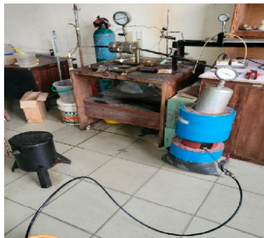
Figure 1. Core Flood set – up (Chemical).
