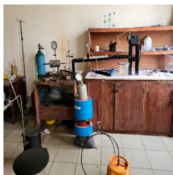
Figure 2. Core Flood set – up (Steam).
