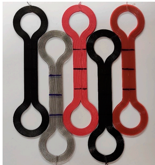
Figure 2. 3D printed specimens reinforced with 5 vol.% metal wires.
