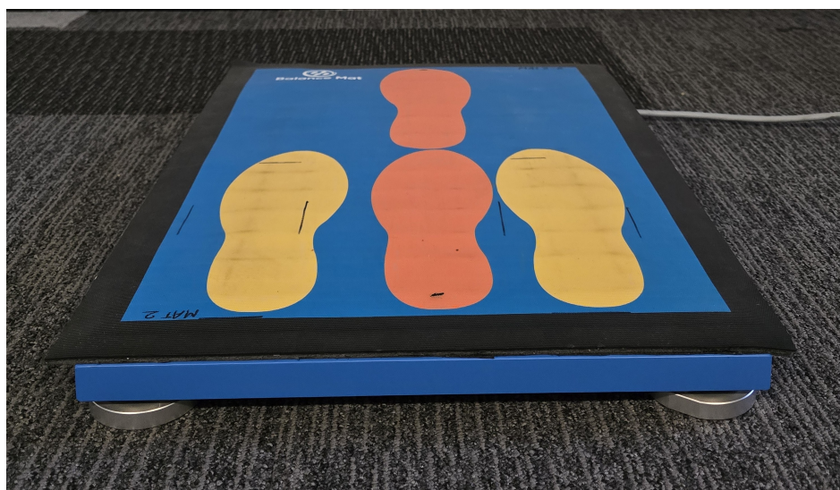
Figure 1. Experimental setup showing the portable Balance Mat positioned on top of the reference laboratory force plate.
