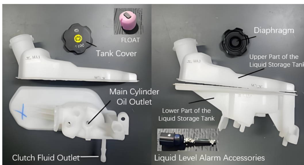
Figure 1. schematic diagram of LST structure.
