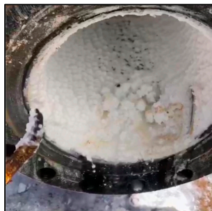
Figure 3. The appearance of silica scale during the use of Inhibitor A.
