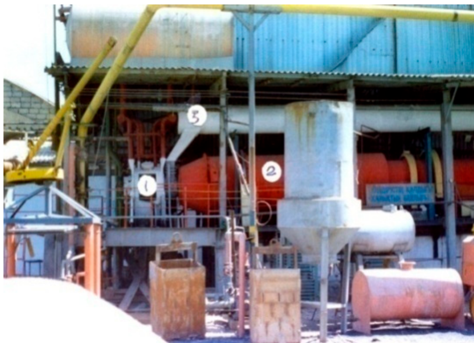
Figure 3. General view of the pilot plant. 1 reactor inversion phase, 2-rotary kiln, 3-bypass.
