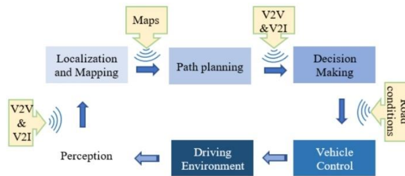
Figure 2. Full autonomous navigation system. Sensor Technology, fusion overview, V2V and V2I [4].
