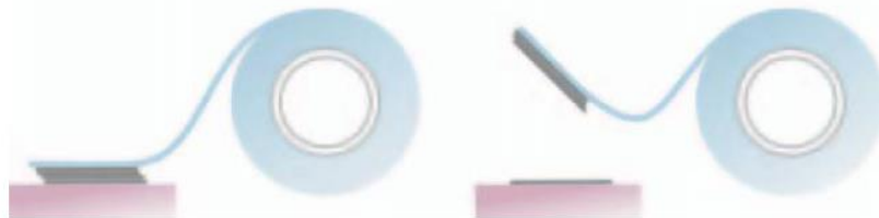
Figure 5. Illustration of the method of obtaining graphene through the micromechanical cleavage of graphite by means of a scotch [21].
