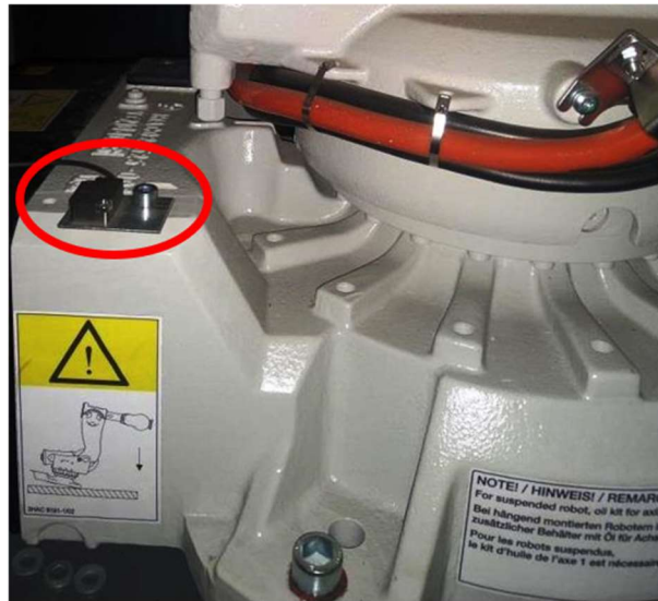
Figure 3. An acceleration sensor (highlighted by the red oval) is mounted on the base of the robot.
