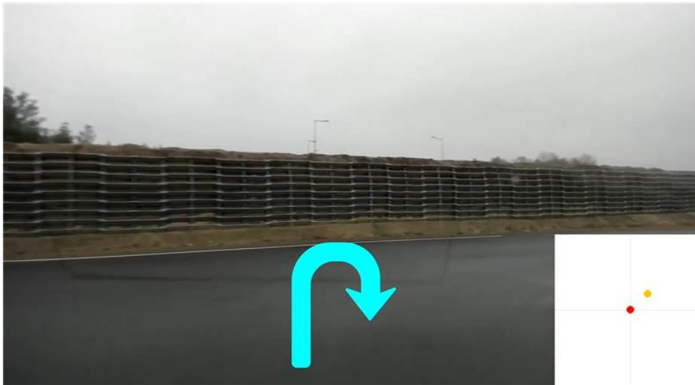
Figure 1. Video HMI maneuver visualization during a sharp right turn. The coordinate grid in the bottom right visualizes the subjects' joystick input (red), as well as the ideal joystick input (yellow, only during test runs).
