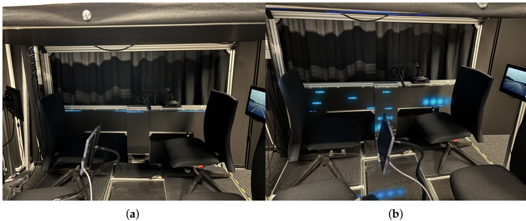
Figure 2. (Side view into the cage. The seats' centres were located at 39 cm above the floor and 34 cm to the side of the nearest side panels. The canopy panels were fixed at 133 cm above the cage's floor. Both images show maneuver visualizations while driving straight. (a) 1D HMI. (b) 2D HMI.
