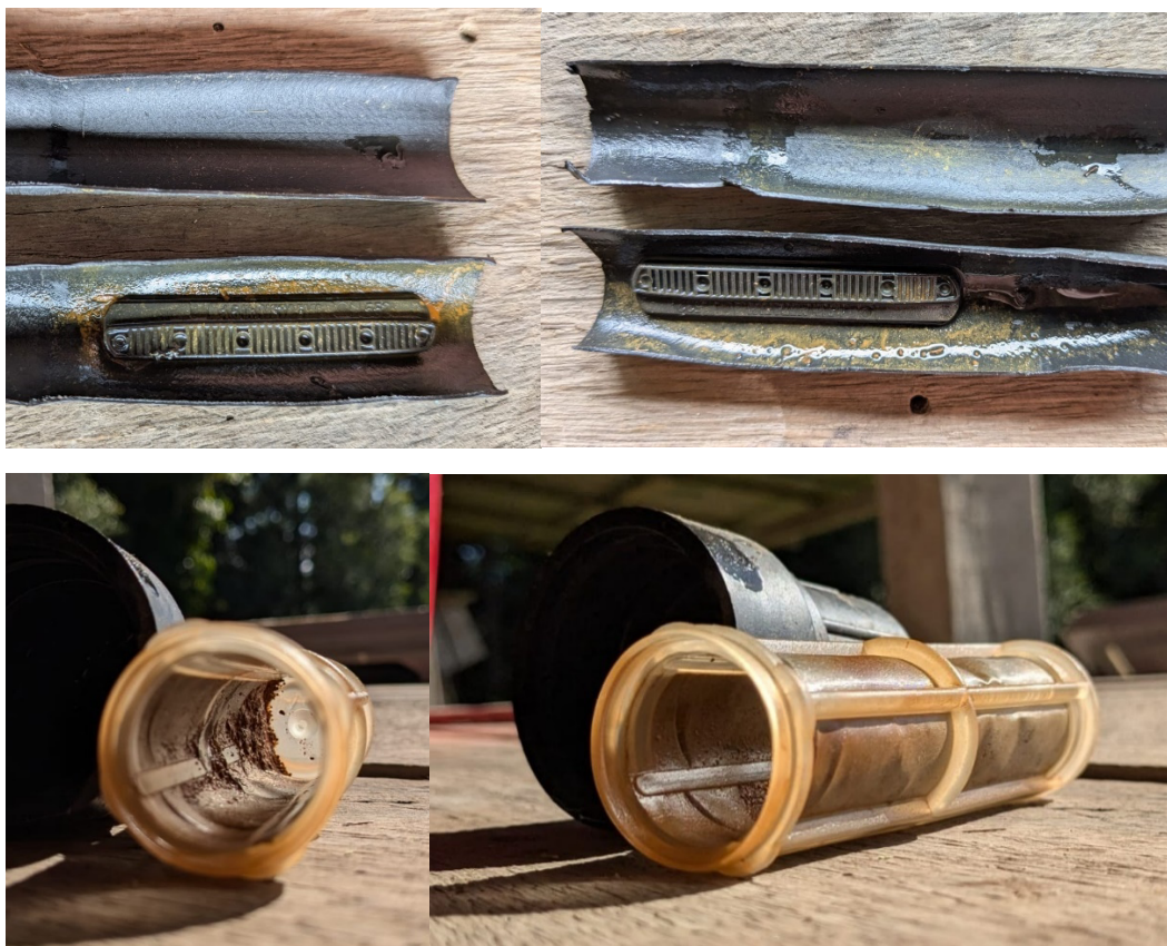
Figure 15. – State of the filter and the last emitters of the lateral line after the end of the tests.
