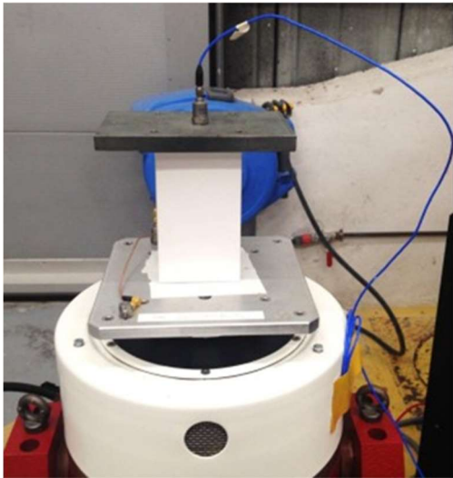
Figure 6. Experimental setup for random oscillation experiment.
