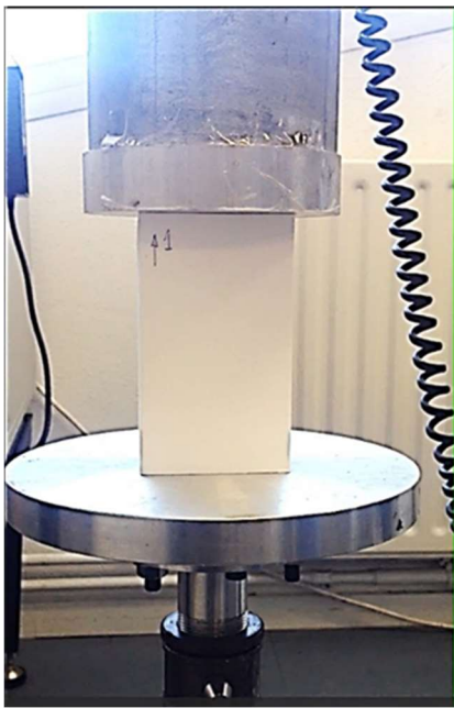
Figure 3. Set up compression test on machine.
