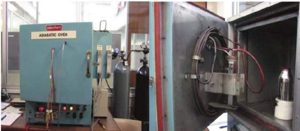
Figure 4. Schematic of adiabatic oxidation reactive apparatus.
