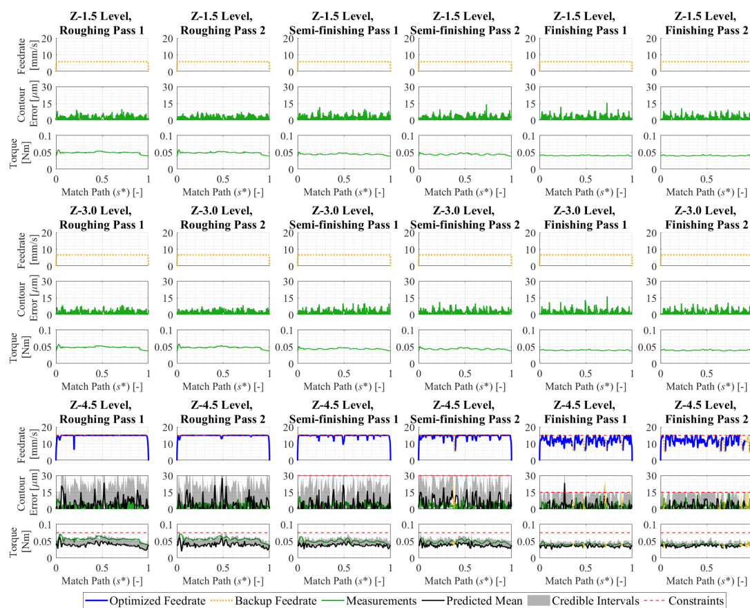
Figure 13. The experimental results of machining tensile test specimen based on feedrate optimization via level-to-level learning. It shows that level-to-level learning does not result in frequent drops in roughing passes due to geometric differences across passes. (Note: the contour error constraints for the roughing passes is 45\mu\text{m} , which is above the plot's axis limit.)
