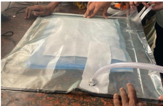
Figure 10. Application of vacuum to remove excess air and compress layers.
