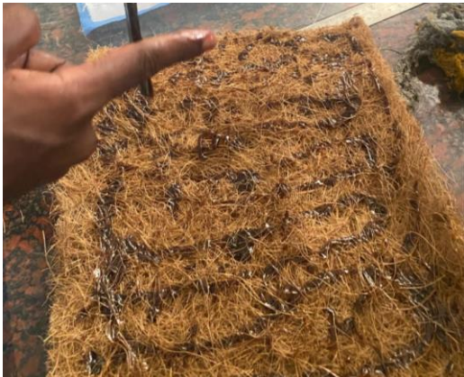
Figure 5. Application of resin (Epoxy+CNSL) onto the coir fiber mat.
