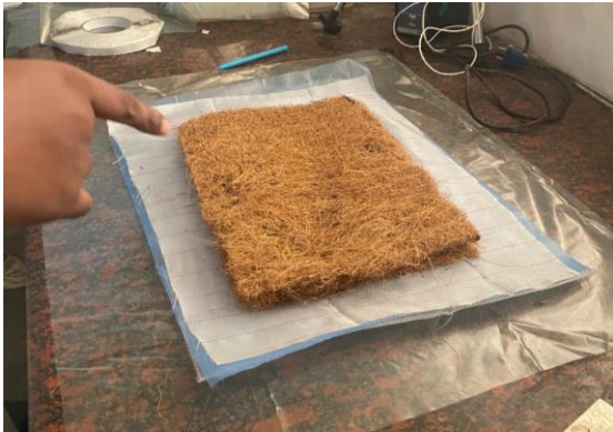
Figure 6. Placement of next coir fiber mat.
