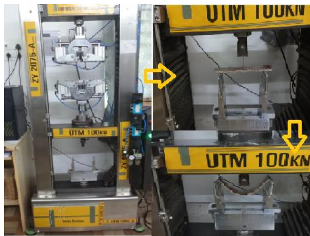
Figure 13. Flexural Testing, This corresponds to the three-point bending test used to evaluate the flexural strength.
