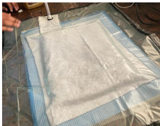
Figure 11. Final Vacuum-sealed setup ensuring proper resin infiltration and curing.
