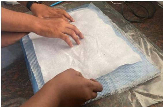
Figure 8. Placement of knitted infusion mesh to allow proper air evacuation.
