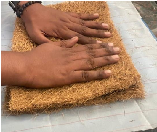
Figure 4. Placement of coir fiber mat on the peel ply sheet.
