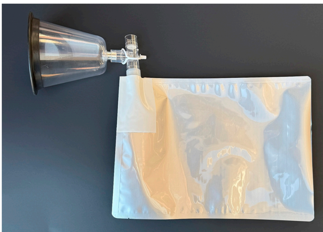
Figure 1. Expired air collection apparatus consisting of a non-rebreathing T-piece connected to a large canine anesthetic induction mask and a 3.79 L mylar food storage bag.
