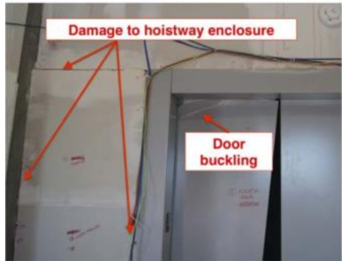
Figure 18. NSE Elevator door damage at a drift ratio of 3.6% [39].
