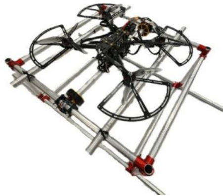
Figure 12. Quadcopter Test Rig for Evaluating the CoM Shifting Mechanism.
