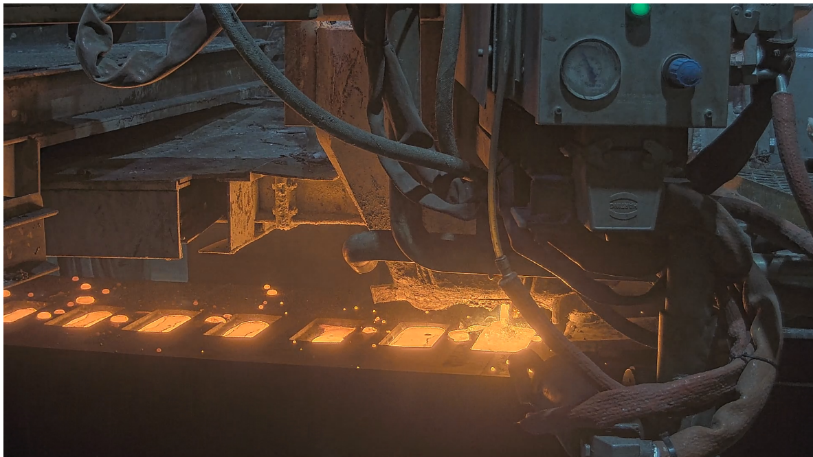
Figure 3. Actual front-view image of the initial section of the vertical sand-casting foundry corresponding to the schematic shown in Figure 2. The image illustrates the operational setup captured in the experimental videos.
