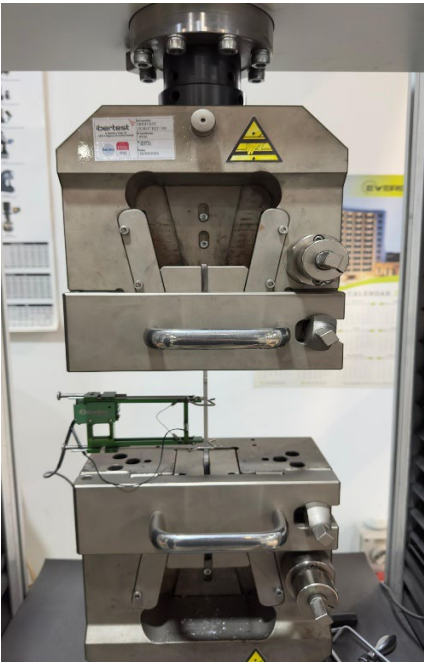
Figure 3. Tensile test set-up of the manufactured AA6061-T6.
