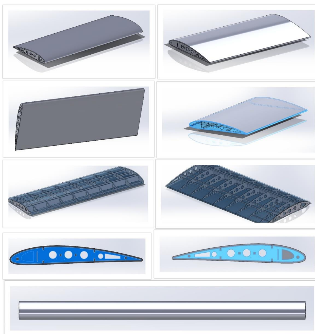
Figure 2-1. SolidWorks rendering of a composite wing with monolithic skin.
