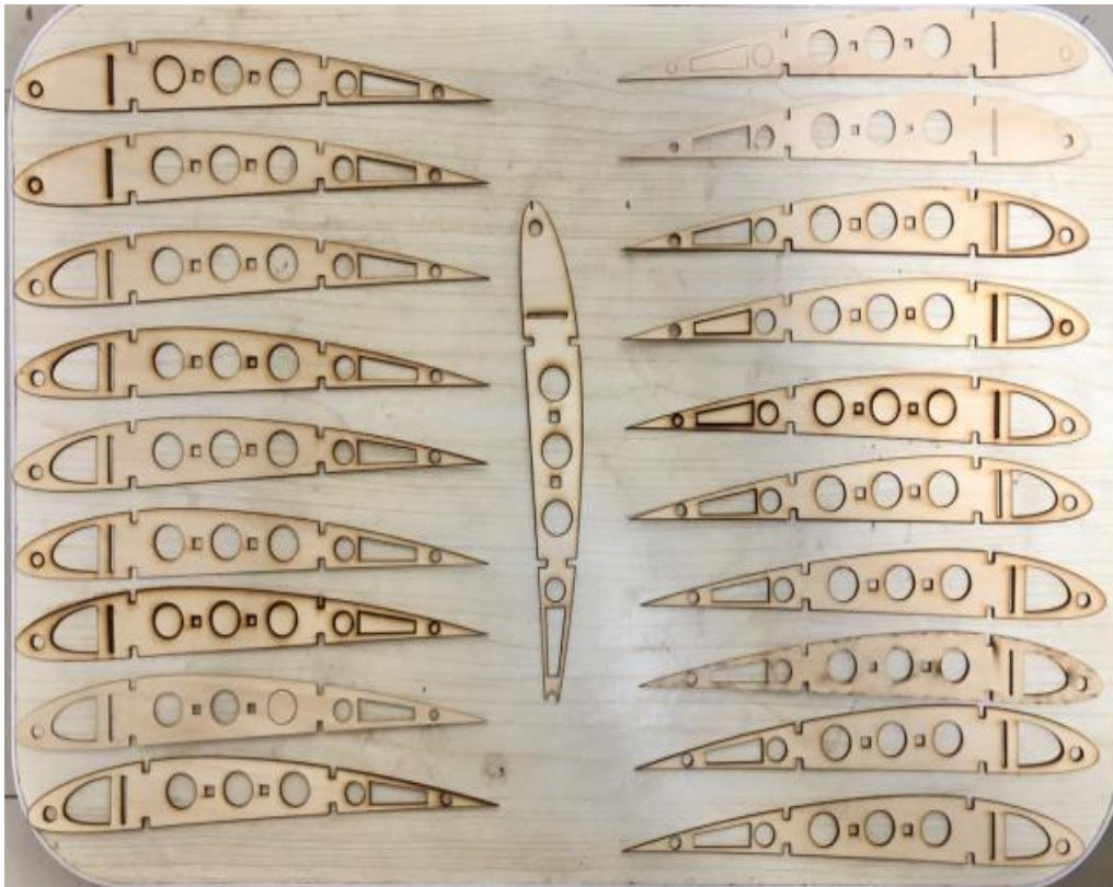
Figure 7-1. Photograph of individual ribs after laser cutting and before assembly.
