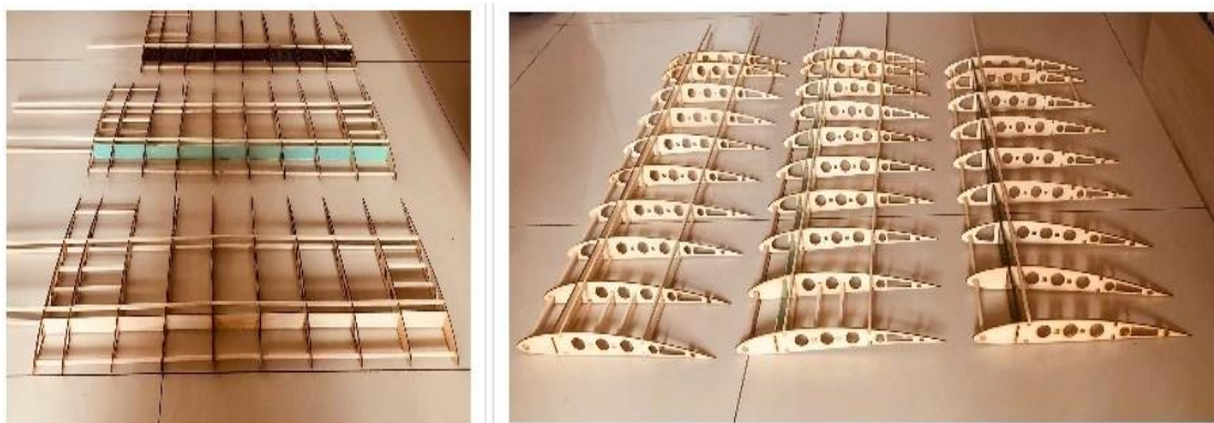
Figure 7-2. Fabricated UAV wing internal structures prepared for future experimental validation.
