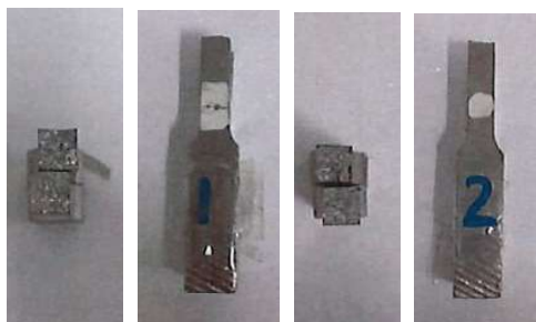
Figure 6. Tensile test specimens of knuckle material.
