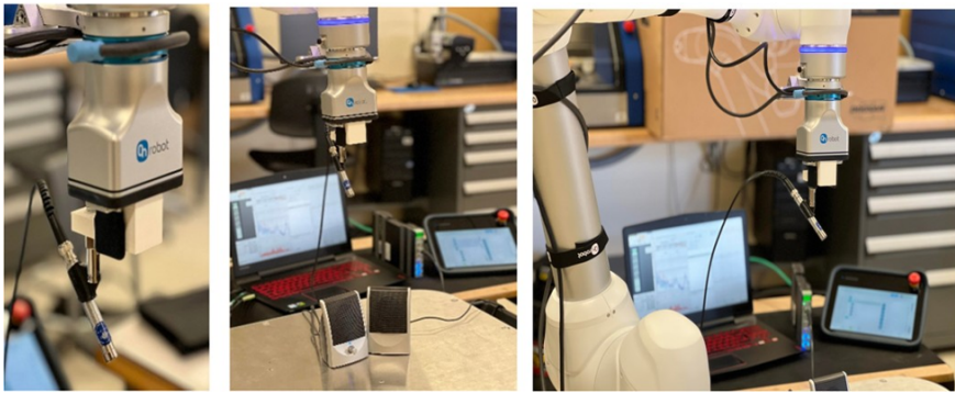
Figure 6. Doosan robot with a microphone following a well-defined trajectory.
