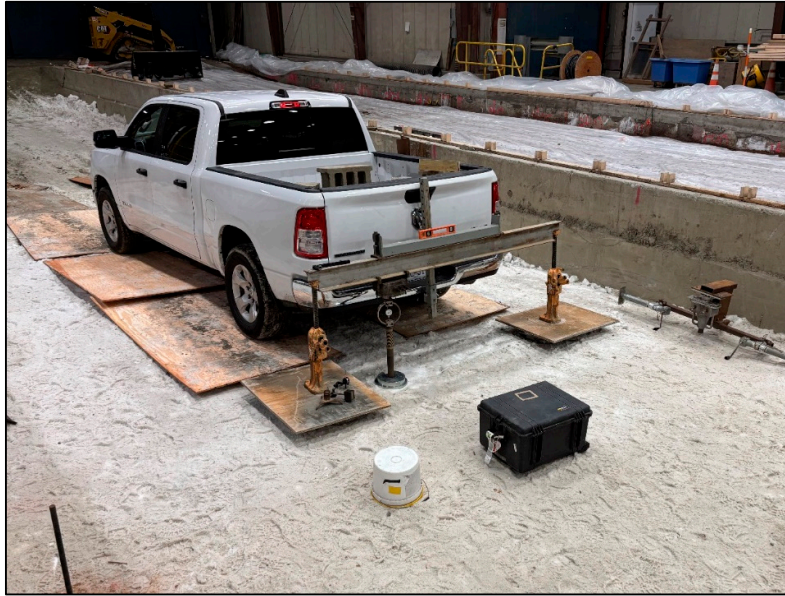
Figure 2. Field CBR setup including the truck with reaction load in the bed, CBR beam, piston apparatus, jacks, base platforms, and plywood sheets used to avoid localized surface disturbance/rutting from the truck tires.
