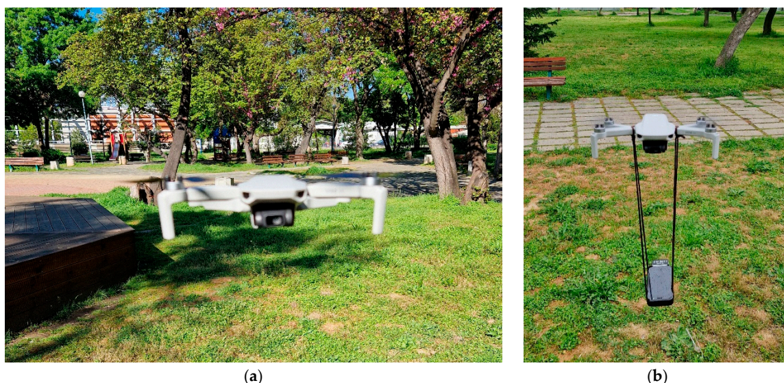
Figure 1. Experimental system and workflow used in the study: (a) DJI Mini 4K during baseline no-payload operation; (b) DJI Mini 4K with the suspended Servo King900 smartphone and attached UTi260M thermal camera.
