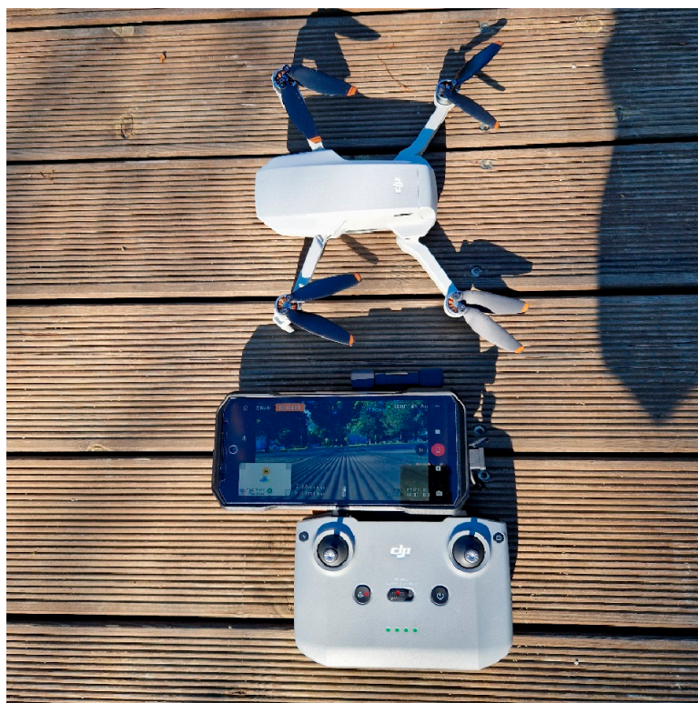
Figure 2. Ground control and monitoring configuration of the experimental UAV thermal sensing workflow. The DJI Mini 4K platform was operated using the remote controller and the Ulefone Armor 27T smartphone, which provided live UAV camera monitoring, telemetry visualization, and screen recording during the field tests.
