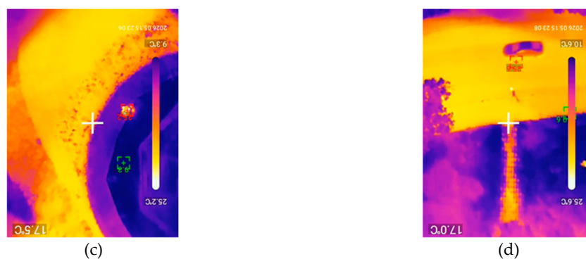
Figure 5. Representative dual-channel comparison between direct thermal-camera output and UAV-recorded smartphone display: (a,c) direct thermal frames recorded by the Servo King900 smartphone with the UTi260M thermal camera; (b,d) corresponding or approximately corresponding UAV RGB frames showing the smartphone-displayed thermal stream during flight. The comparison demonstrates that the direct thermal stream provides clearer thermal information, while the UAV-recorded display remains usable for preliminary monitoring despite payload oscillation, reduced sharpness, display-related effects, and indirect optical acquisition.
