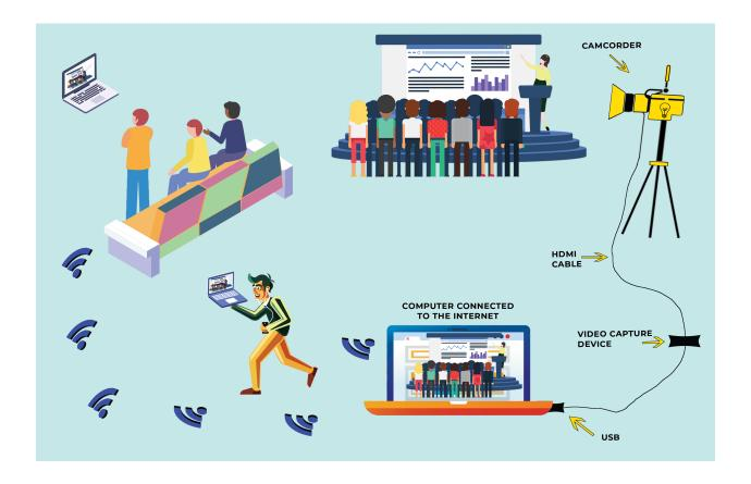
**Figure 1. Schematic of the basic live video streaming equipment set up.** Illustration by Moema Umann.
