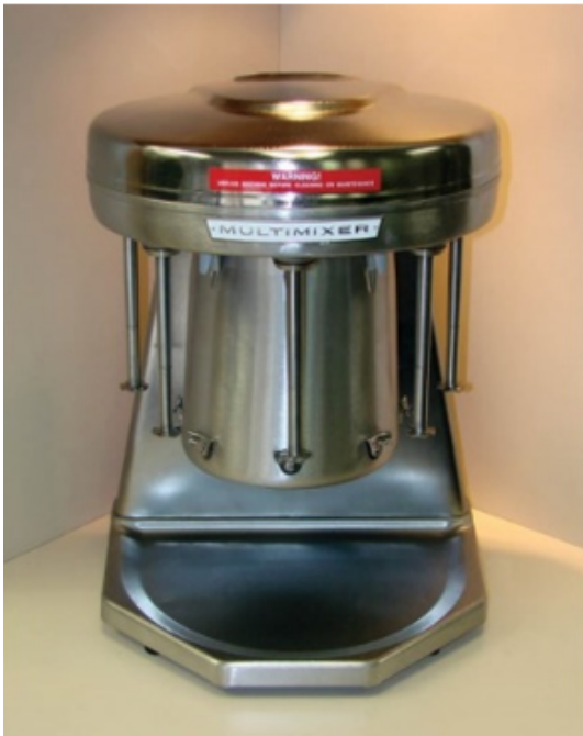
Figure 4. Multimixer from Sterling Multi Products, Inc., model 9B5CH1 used to generate bentonite mixtures.
