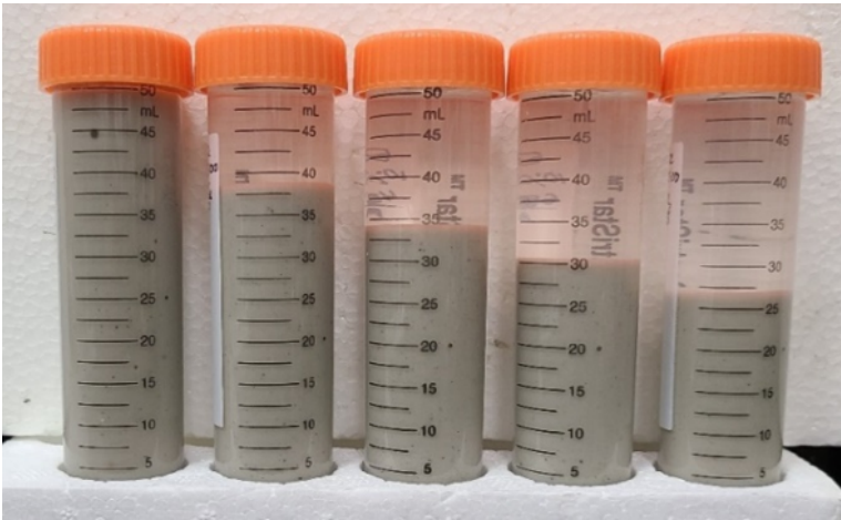
Figure 5. 10% QG dispersed in 2,3,4,6, and 12 g CaCl 2 per liter of distilled water. Picture was taken after a constant degree of dispersion was achieved at the infinite time limit.
