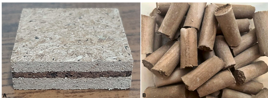
Figure 3. Proposed uses to stranding Sargassum in Brazil, as (A) composition panels [33] and (B) ceramic addition [31].
