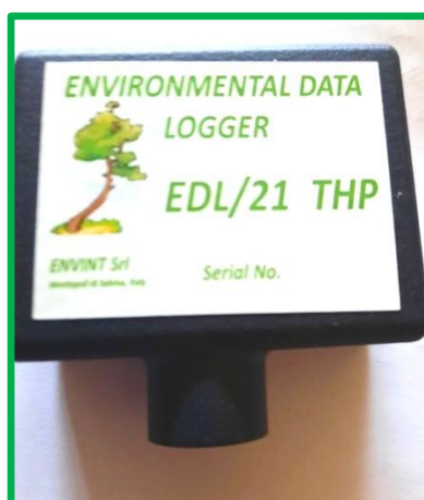
Figure 4. Datalogger used in the campaign. Dimensions: 7x4.5x2.3 cm.
