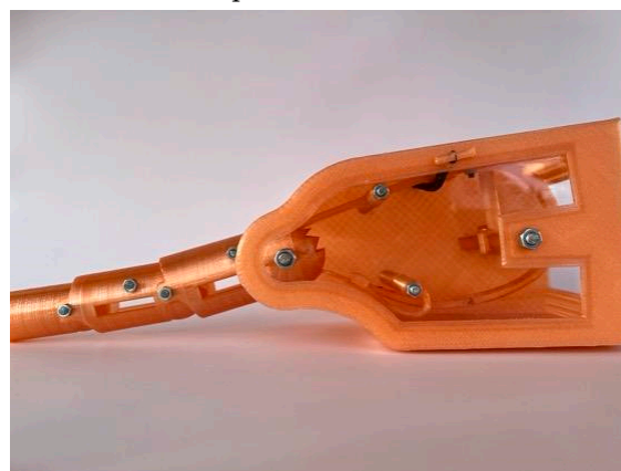
Figure 6. Optimized model of the reconstruction of the index finger of the second “Iron Hand”.
