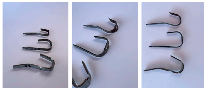
Figure 12. Presentation of the results from different perspectives: the 0.75 mm thick spring on the left, the 1.2 mm thick spring in the middle, and the 1.8 mm thick spring on the right.
