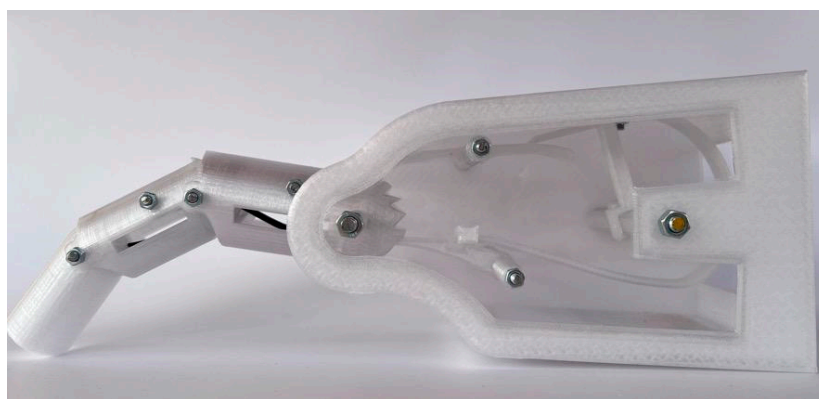
Figure 4. 3D-printed model of the index finger of the second “Iron Hand” at a scale of 2:1.
