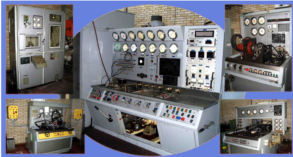
Figure 9. Universal test stand AMS ZI 108-94262 TYPE BAH 1622/B38-5 (3x380V, 50Hz, 100 KW).
