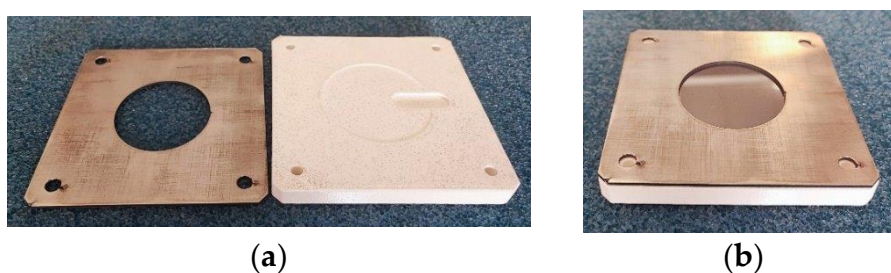
Figure 5. Field-deployable soiling sampler (a) open position, (b) sampler containing a silicon wafer for FTIR characterization.
