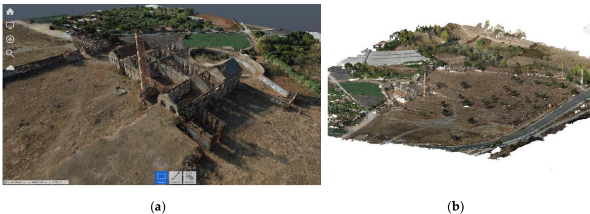
Figure 9. Digital point-cloud: (a) Main building in Autodesk ReCap; (b) General view in Autodesk Revit.
