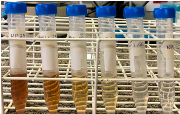
Figure 1. Reaction tubes containing suspensions of AgNPs, synthesized using varying concentrations of soybean leaf aqueous extract: 25, 12.5, 6.25, 3.12, 1.56, and 0.78 mg mL -1 , respectively.
