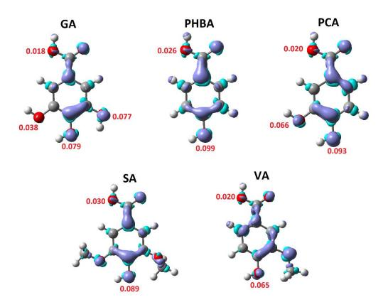
**Figure 4**. Isosurface plots of fukui function  $f^0$  and condensed values at hydroxylic O atoms.
