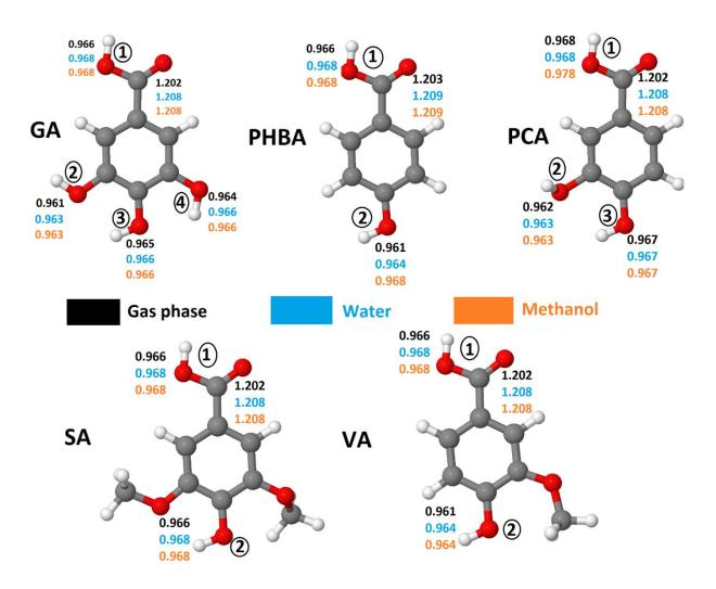
**Figure 1**. Optimized geometries of the antioxidants considered in this study. Bond lengths in Å computed at the M06-2X/6-311++G(d,p) level
