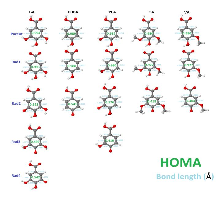
**Figure 2**. HOMA and bond lengths of the parent and radical resulting from the homolytic rupture of O-H bonds from GA, PHBA, PCA, SA and VA.
