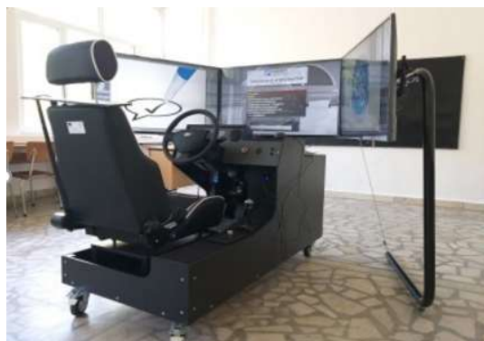
Figure 7. Driving simulator used to measure driver reaction time.
