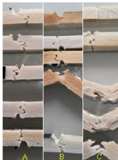
Figure 11. Some fracture profiles of intact specimens. 11A) 40%, 11B) 50% and 11C) 60% fiber theoretical volume fraction.
