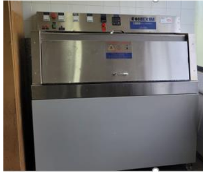
Figure 3. C-UV accelerated aging system from ADEXIM-COMEXIM manufacturer [22].
