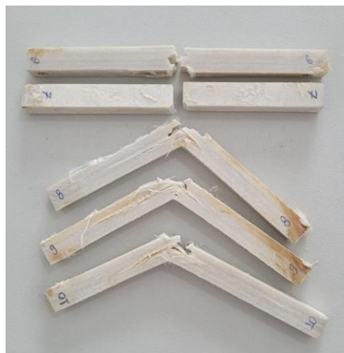
Figure 9. Some fracture surface profiles of intact specimens with 60% of theoretical volume fraction.
