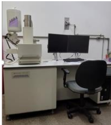
Figure 4. Shimadzu SSX550 Scanning Electron Microscope used to characterize the fracture surfaces.
