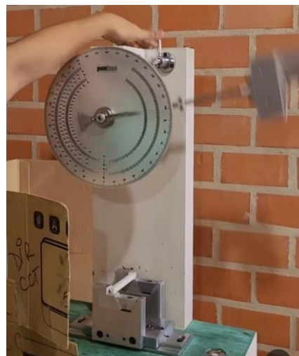
Figure 2. Impact test equipment used in the experiments with the laminate specimens [22].
