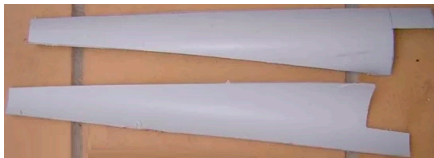
Figure 18. Manufactured wind turbine blades.
