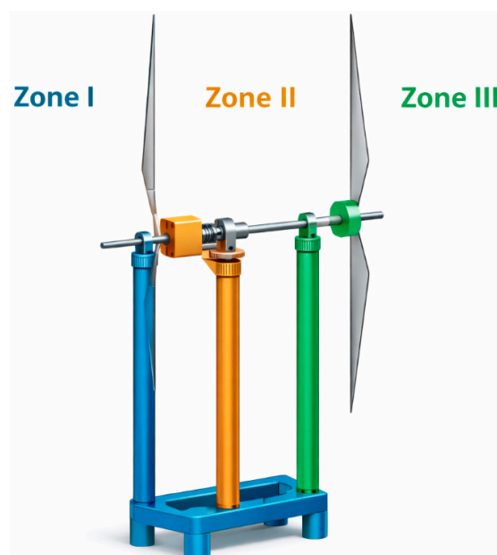
Figure 5. Zones of the air flow location at interaction with wind wheels.
