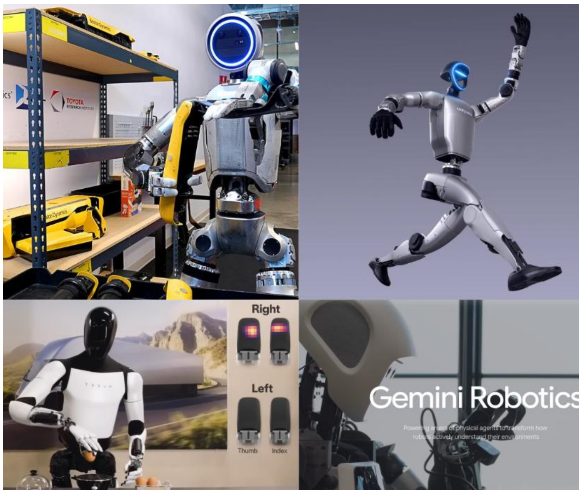
Figure 11. Industrial VLA-powered humanoid robot systems. (a, top left) Boston Dynamics Atlas with TRI Large Behavior Model performing warehouse manipulation [186]. (b, top right) Unitree humanoid executing dynamic whole-body control. (c, bottom left) Tesla Optimus humanoid with dexterous hands for general-purpose manipulation [187]. (d, bottom right) Google DeepMind Gemini Robotics, which integrates actions as a native Gemini modality for dexterous manipulation and general-purpose robot control [178]. Figures obtained from the respective organizations.
