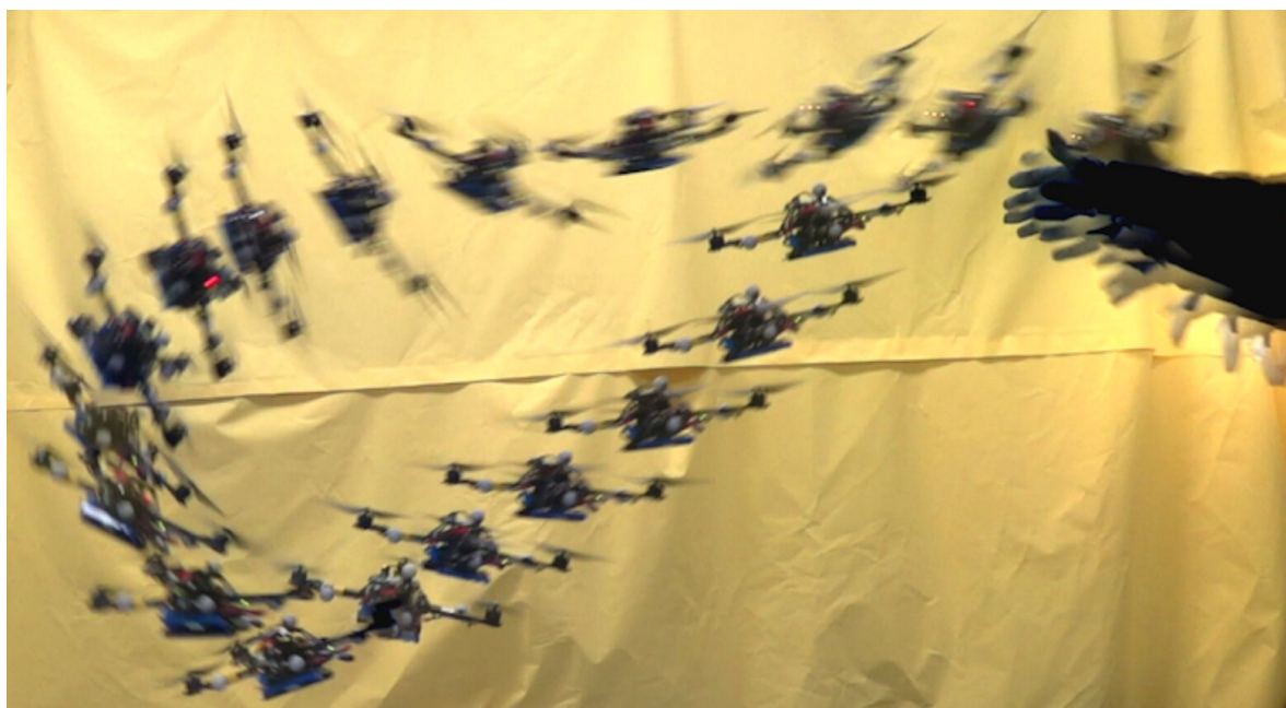
Figure 7. An RL-trained quadrotor recovering from an inverted throw at 5 m/s. The policy maps state to motor commands at 7\ \mu\text{s} per step, establishing the viability of learned end-to-end drone control. Figure obtained from Hwangbo et al. [136].
