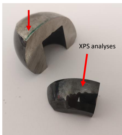
Figure 8. Red arrows indicate the place of XPS analysis on worn surface of retrieved.
