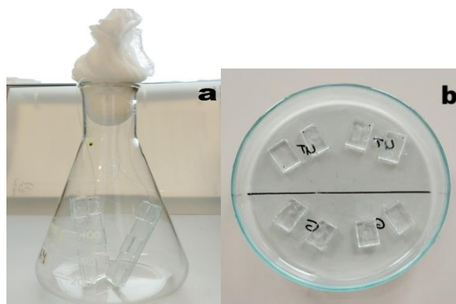
Figure 1. Erlenmeyer flask (a) and glass Petri dish (b) with coupons before the addition of algal suspension.
