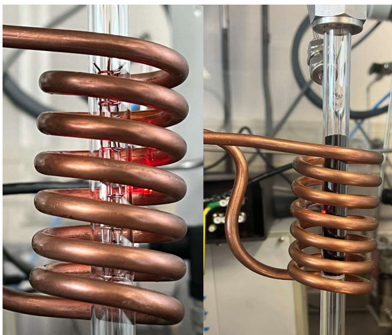
Figure 5. Close up pictures of the quartz reactor with just the workpiece inside (left) and with the catalyst added (right) inside of the induction heating coil.
