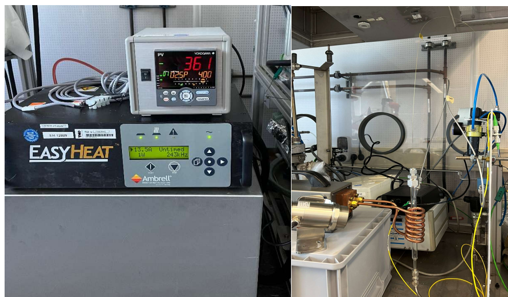
Figure 3. Photo of the induction heating experimental setup.
