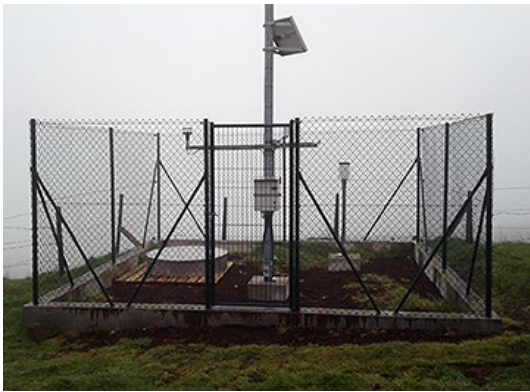
Figure 3. Alto do Cabouco meteorological station located on Faial (Azores). The station belongs to the regional hydrometeorological monitoring network and provides observations of wind speed and wind direction, which were used to characterize atmospheric transport conditions influencing the variability of NO 2 in the study area.
