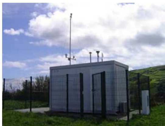
Figure 2. Location of the Espalhafatos air quality monitoring station on Faial (Azores), used for continuous measurements of NO 2 and PM 10 under rural background conditions. The station is part of the regional air quality monitoring network and contributes data to the national air quality information system QualAr.
