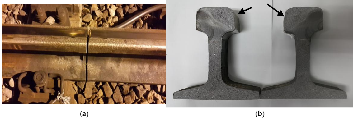
Figure 2. Rail fracture status: (a) overview of rail fracture; (b) gauge corner fracture.
