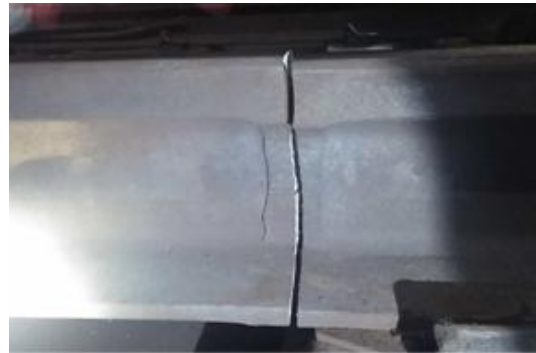
Figure 20. CWR weld fracture near ventilation shaft.
