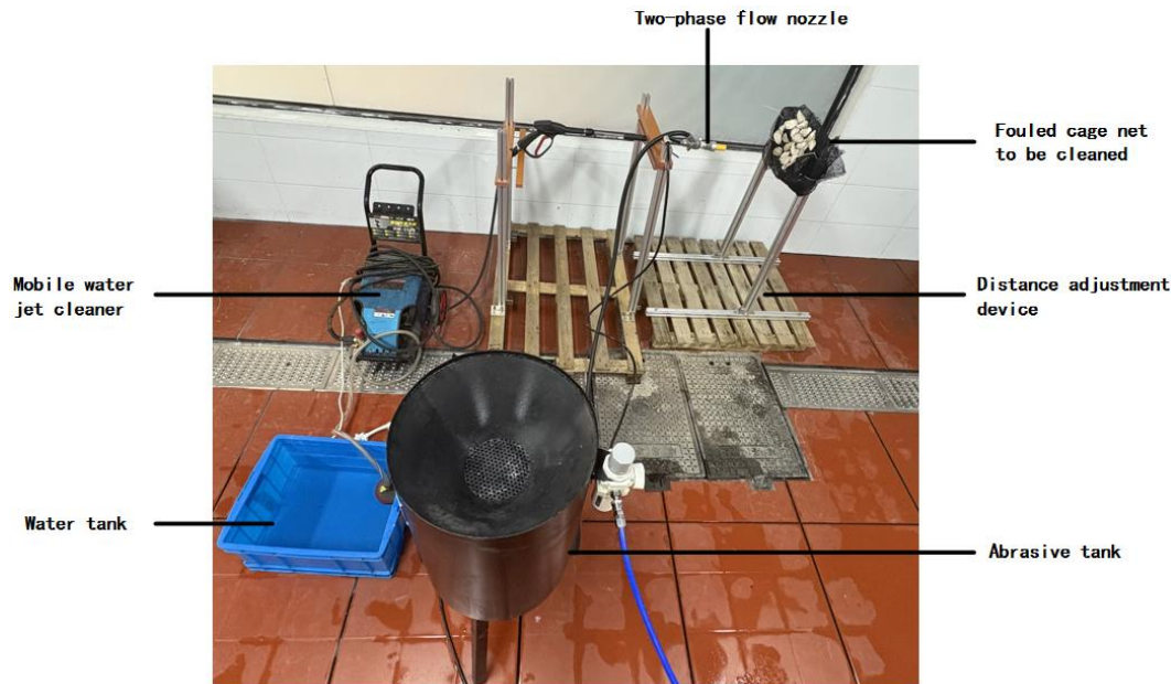
Figure 15. LPAWJ cleaning test platform.
