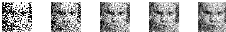
Figure 4. The superimposed images of the grayscale image "disgust" composed of spikes obtained by the Poisson encoder.
