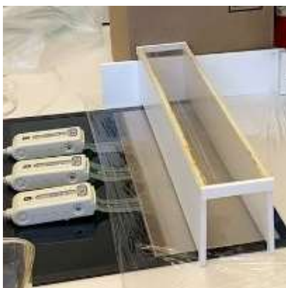
Figure 7. The gait testing unit comprised of the Tekscan pressure sensor mat (black) that was modified to include a tinted Plexiglas tunnel (width 17.0 cm, height 17.0 cm, length 44.7 cm) for the purpose of guiding the rats across the mat and a goal box. .
